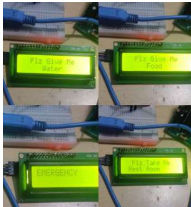
Figure3: Messages displayed on LCD
