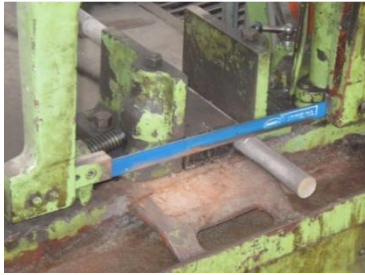
FIGURE: 1 Cutting of work piece by power saw as per reference paper.
