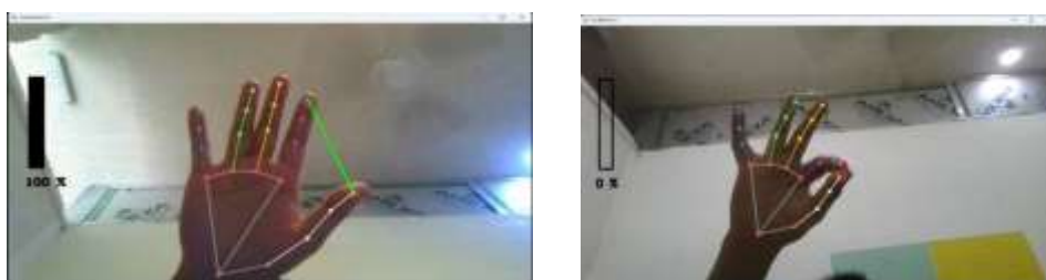
Fig. 6 – (a) Volume 100% [Distance between index and thumb]; (b) Volume 0% [Mute]
