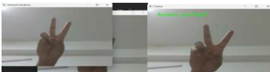
Fig. 10 – (a) Capturing hand pattern for recognition [Press “c” to capture]; (b) Hand-pattern Recognized [Access Granted]
