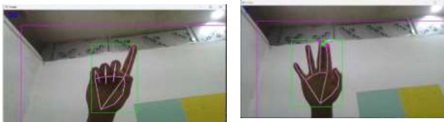
Fig. 7 – (a) Movement of the cursor using index finger; (b) Left Click [Tapping the index & the middle finger]
