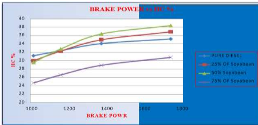
Brake power Vs (HC %) in case of soyabean biodiesel blends
