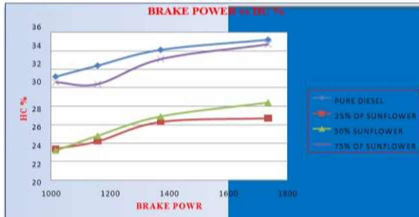
Brake power Vs (HC %) in case of sunflower biodiesel blends blends with biodiesel
