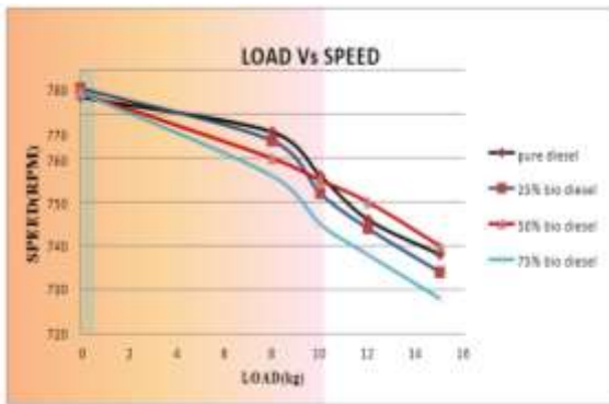
Variation of speed with load for pure diesel and diesel blends with biodiesel (Soyabean and Sunflower)
