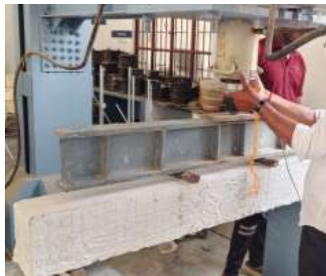
Figure 3: Experimental Setup of Beam in the Loading Frame
