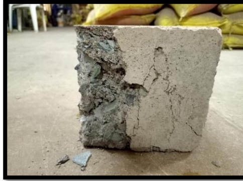
Fig. No. 05 Green concrete cube specimen
