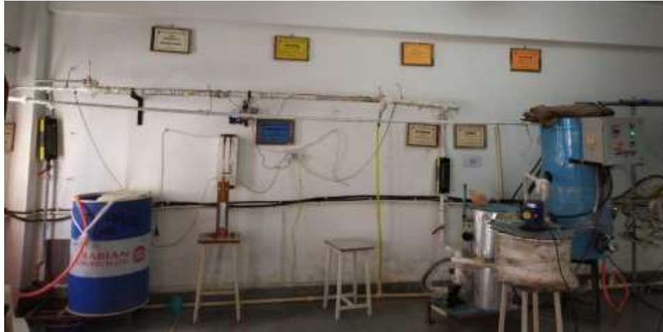
Fig 3.1:- Experimental set-up for Double Pipe Type Heat-exchanger available in HMT Lab
