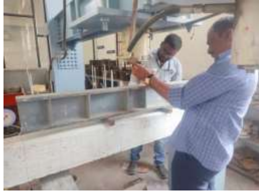
Fig. 10 – Experimental setup of the RC beam in loading frame
