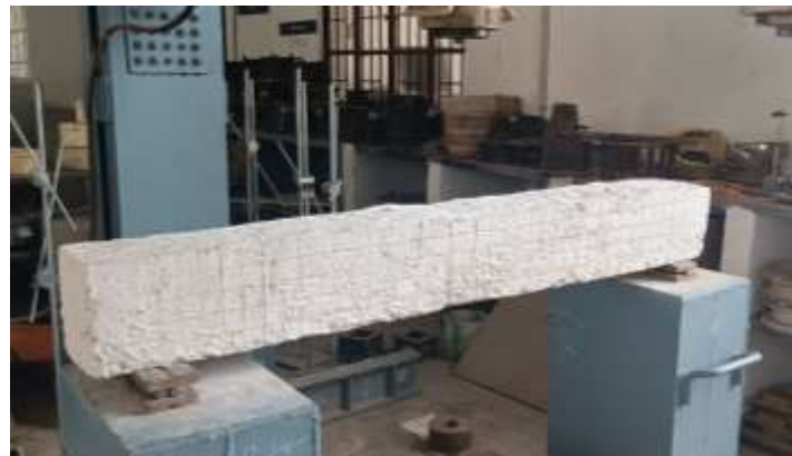
Fig. 7 - Experimental Setup of Beam in Loading Frame
