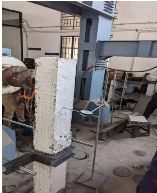
Fig 16: Test setup of Half gouted sleeve column specimen
