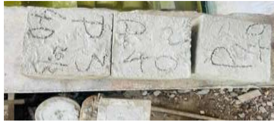
Fig 8: M40 grade Cubes for split bond test
