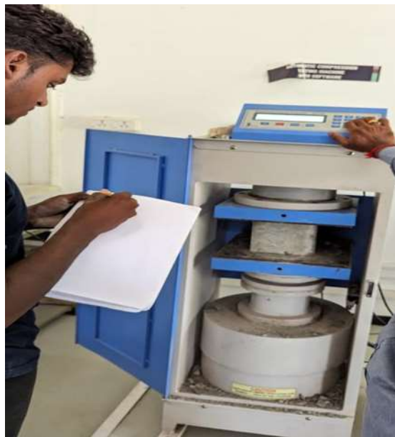
Fig 9: Testing of M40 grade Cubes for split bond test
