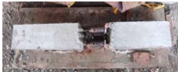
Fig 6: casting of Half grouted sleeve in column-to-column connection.
