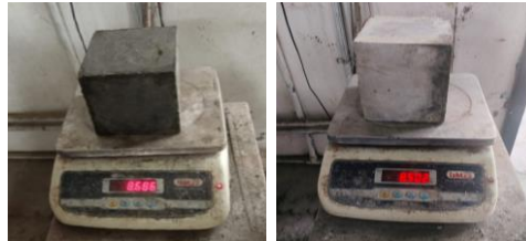
Fig.4. Water absorption test
