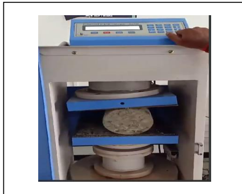
Fig.2. Split tensile strength test
