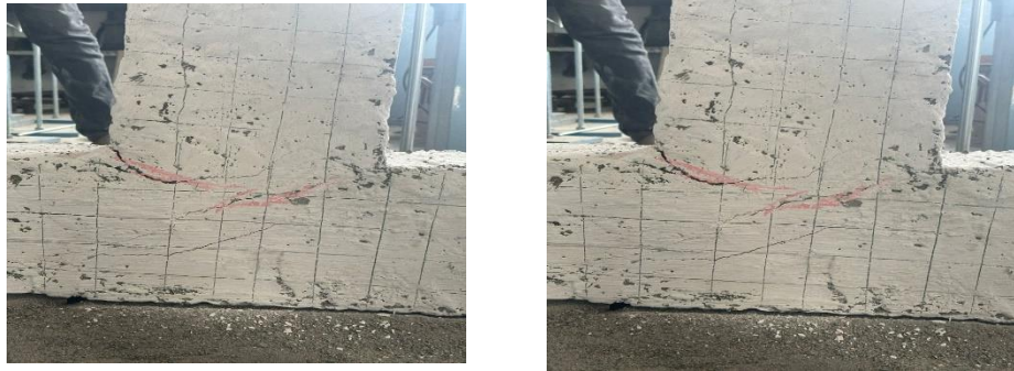
Fig11. Cracks developed in lap joint and grouted sleeve joint
