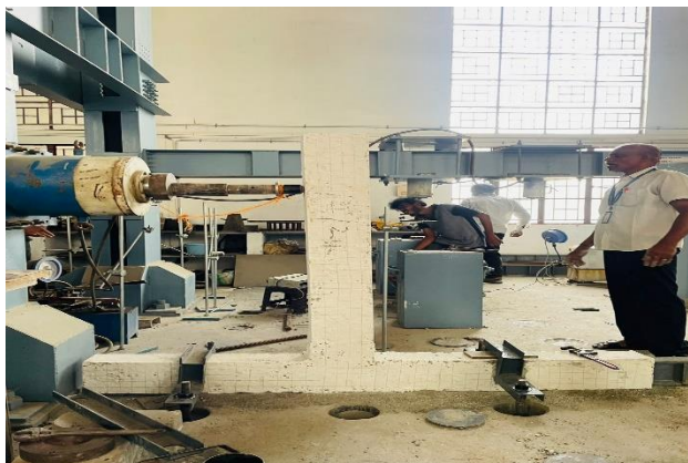
Fig10. Test Setup for lap joint and grouted sleeve joint
