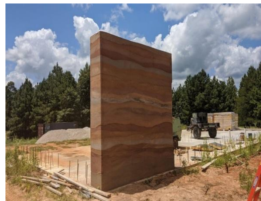
Fig. Developed slammed soil wall panel
