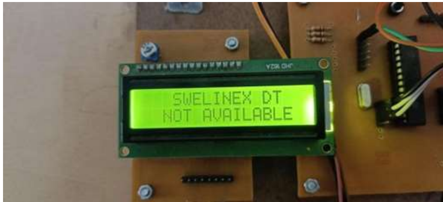
FIG 4.2: LCD Screen Displaying Medicine Out of Stock
