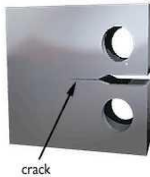
Figure: Fractured test specimens
