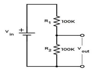
float voltage = (((val \* 3.3) / 1024) \* 2 + calibration); //multiply by two as voltage divider network is 100K & 100K Resistor float bat\_percentage = map(voltage, 2.8, 4.2, 0, 100); float temp = ((val \* 1.3) \* 3.3) / 1024.0;
