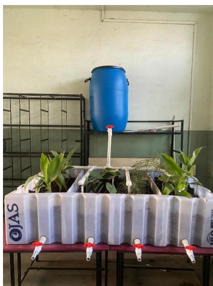
Fig.1.2: Vertical Flow Construction Wetland Prepared Model
