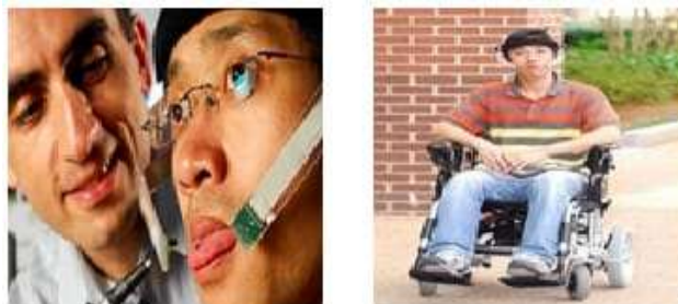
Fig.1: Tongue Drive System based on magnetic tracer.
