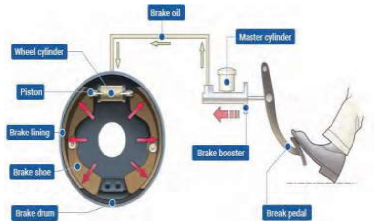
Fig 2: working principle of a brake drum
