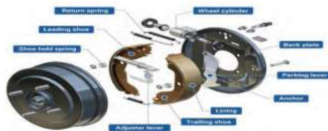
Fig 1: Brake drum and its parts
