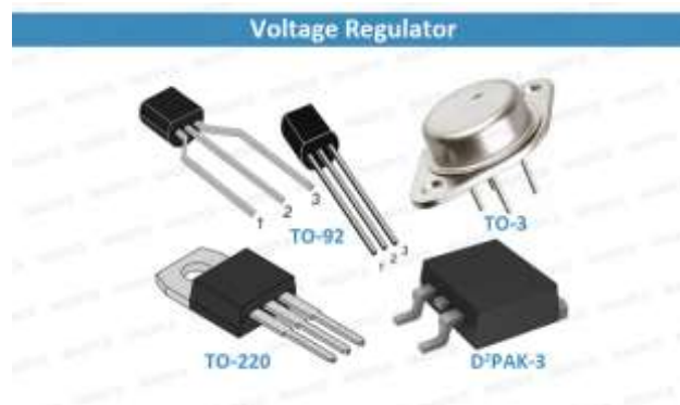
Figure-3 Voltage Regulator
