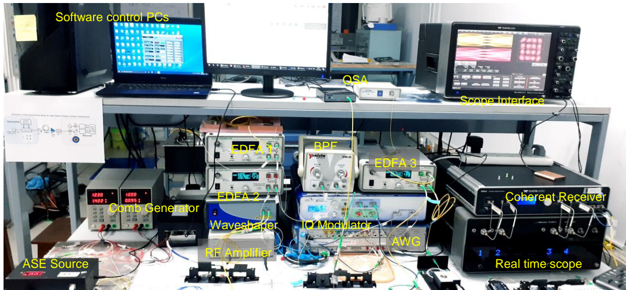
Fig. 3. Experimental setup for the generation, transmission and reception of optical superchannel signals.
