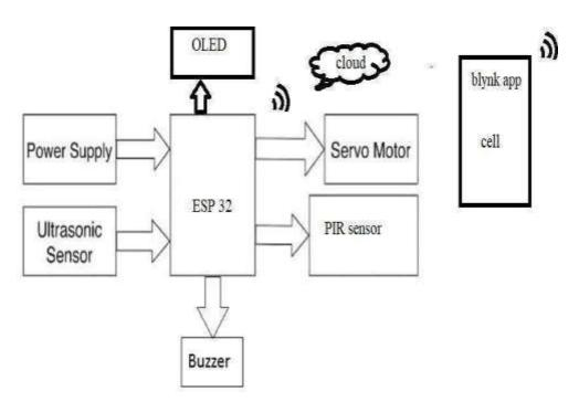
**Ultrasonic Sensors:** These sensors emit sound waves at frequencies beyond the range of human hearing. When these waves encounter an object or individual, they bounce back and are detected by the sensor. By measuring the time it takes for the sound waves to return, the sensor can calculate the distance to the object and its position
