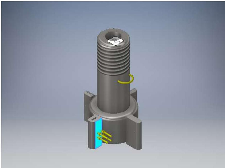
Fig1.0(a). Gas Impeller Model with Constraint, Turning Moment and Gas Pressure
