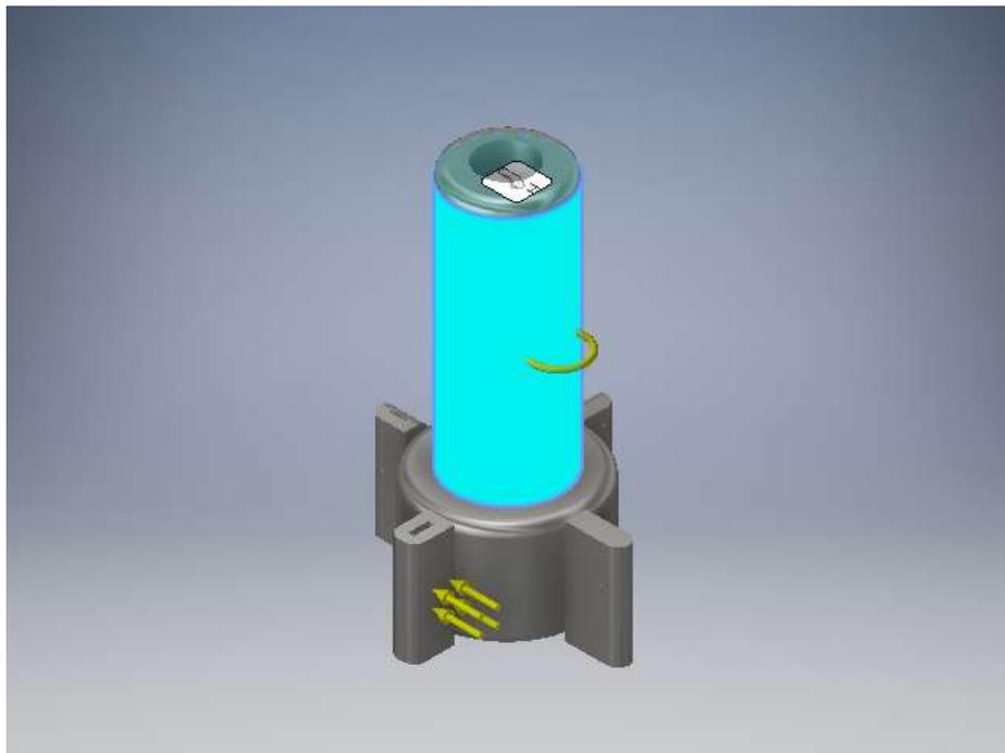
Fig1.0 (c). Gas Impeller Model with Constraint, Turning Moment and Gas Pressure
