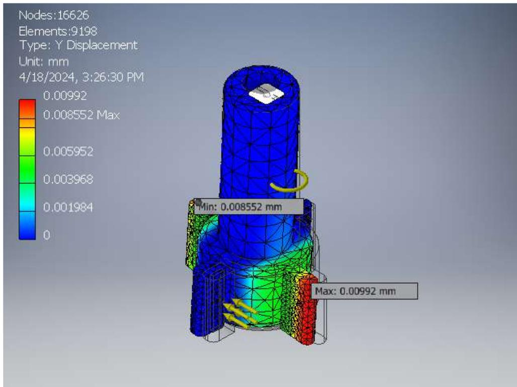
**Fig 5.0(b). Maximum Displacement**
