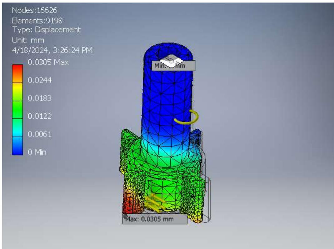
Fig5.0(a). Maximum Displacement
