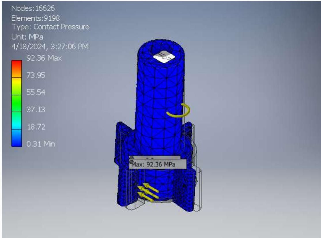
**Fig7.0. Maximum Contact Pressure**
