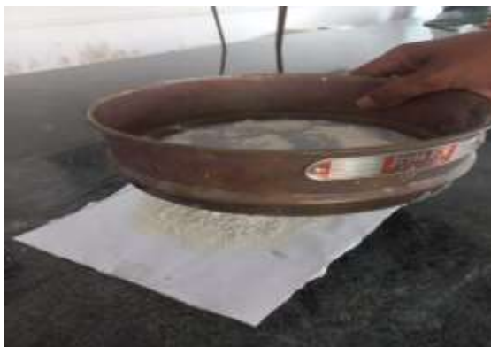
(Prepared dusting powder passing through sieve number-120)
