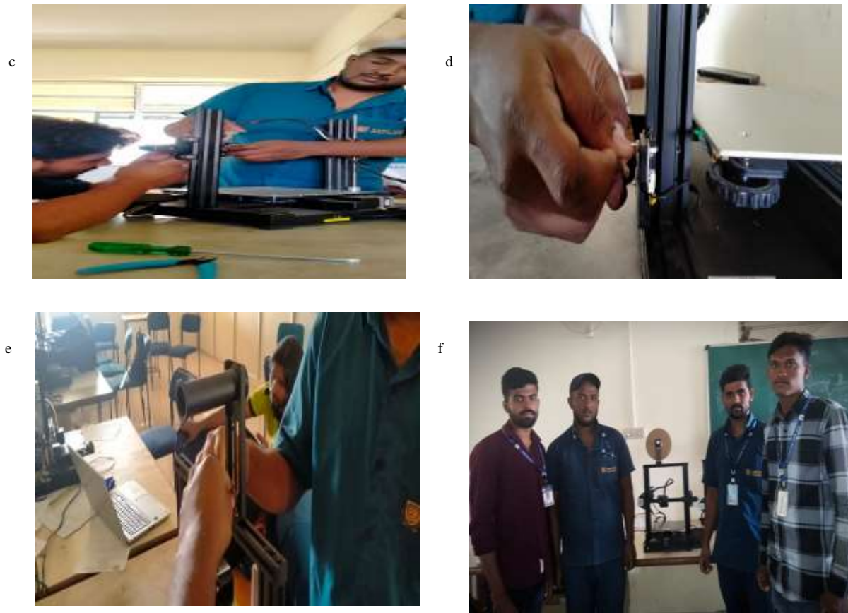
Fig 2- (a) Assembly of LCD screen display, (b) Assembly of extruder kit, (c) Assembly of frame, (d) Assembly of Z axis sensor, (e) Assembly of filament holder (f) final Assemble of Ender 3 v2 3D printing machine .
