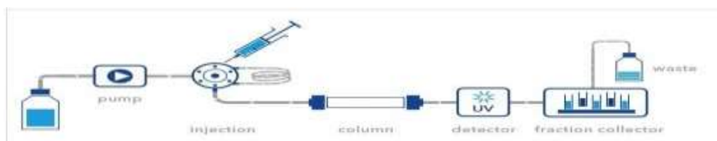
Fig 1 instrumentation Of preparative high performance chromatography Reservoir
