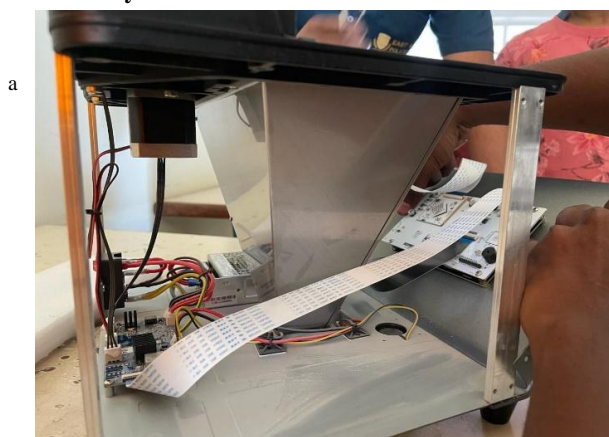
Fig 1- (a) Touch screen display, (b)Build platform , (c) 8K mono LCD display, (d) Mother board, (e)FEP film & VAT gasket , (f) Stepper Motor.
