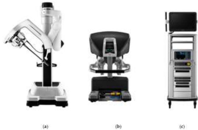
Figure 11. Da Vinci robotic surgical system [60]. (a) Patient cart. (b) Surgeon console. (c) Vision cart.
