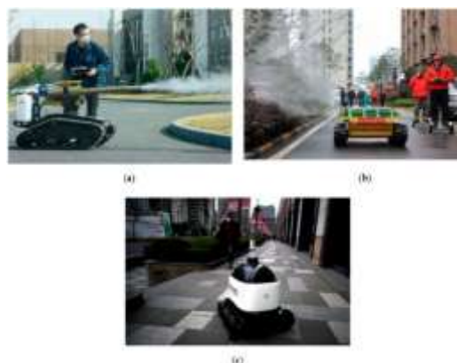
Figure 10. Spraying and sanitizing robots in residential areas of China [58]. (a) Remote control disinfecting mobile robot in Hangzhou, China. (b) Spraying robots to disinfect large residential areas in China. (c) A hand sanitizer-dispensing robot in Shanghai.
