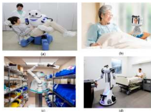
Figure 5. Nursing robots in hospital and at home for elderly care. (a) Robear—a robotic bear nurse to lift patients in Japan [33]. (b) Dinsow robot for elderly entertainment and face-to-face calls [34]. (c) Moxi—nursing robot placing medicines in bins [35]. (d) Robot attendant for hospital care [36].
