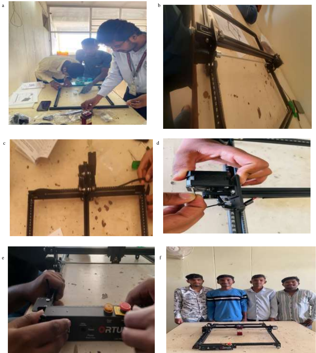
Fig 2- (a) Assembly of Laser Frame, (b) Assembly of X-axis Assembly, (c) Assembly of Timing belts , (d) Assembly of Stepper Motors, (e) Assembly of Mainboard (f) final Assemble of Laser engraving machines
