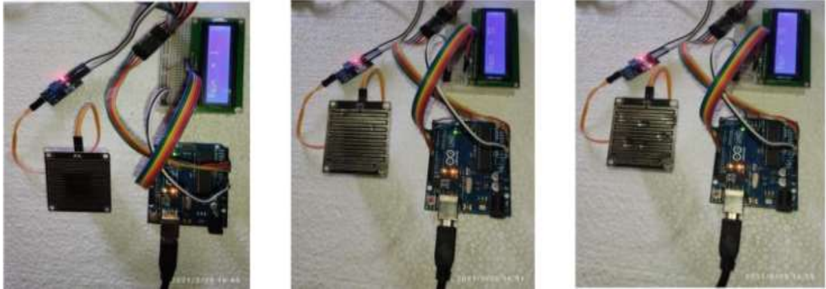
Figure 4.2 RAIN SENSOR TESTING
