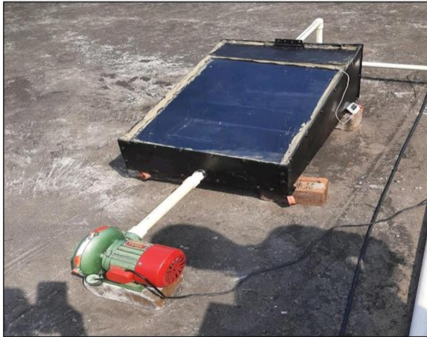
Figure 2. Roof top unit with baffles and stones
