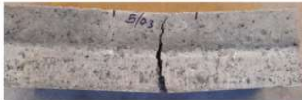
Figure 5 Failure of fiber reinforced concrete
