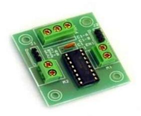
L293D is a typical Motor driver or Motor Driver IC which allows DC motor to drive on either direction. L293D is a 16-pin IC which can control a set of two DC motors simultaneously in any direction. It means that you can control four <u>DC motor</u> with a single L293D IC.
