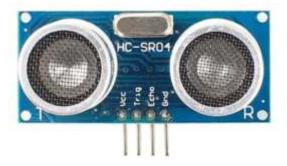
An ultrasonic sensor is a sensor that measures distances through ultrasound which travels through the air. If the ultrasound hits an object or obstacle on its path, it will then bounce back towards the sensor. One of the most popular ultrasonic sensors would be the HC-SR04. The configuration pin of HC-
