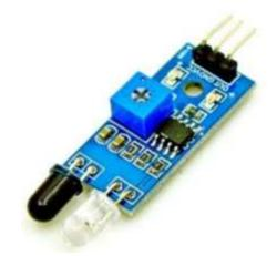
Infrared (IR) sensors are devices that detect or measure infrared radiation in their surroundings. IR sensors work based on the principle that all objects emit some level of infrared radiation. These sensors detect this radiation and convert it into an electric signal, which can then be processed.
