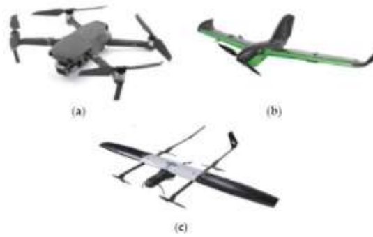
Figure 1. Different types of UAV: (a) rotary wing, (b) fixed wing, (c) fixed-wing hybrid [35].
