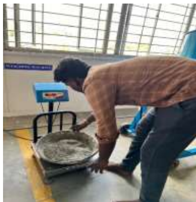
Fig 1: weighing of cement
