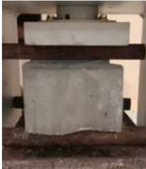
Figure 4 Flexural Strength Test (Mahdi et al. 2022)
