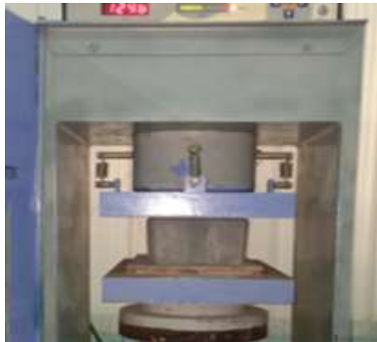
Figure 2 Compressive Strength Test (Mahdi et al. 2022)
