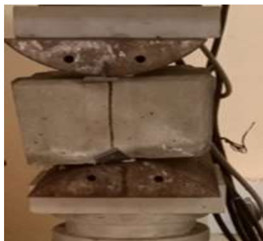
Figure 3 Splitting Tensile Strength Test (Mahdi et al. 2022)
