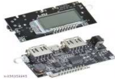
Figure 10: Power Bank Module
