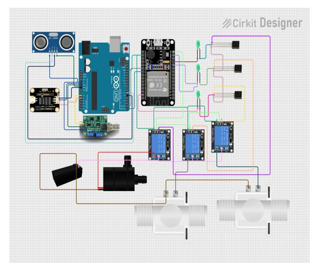
The core of the system involves the utilization of an ESP32 Microcontroller and an Arduino Uno. These components serve as the brains behind the operation, orchestrating the entire system's functionality.
