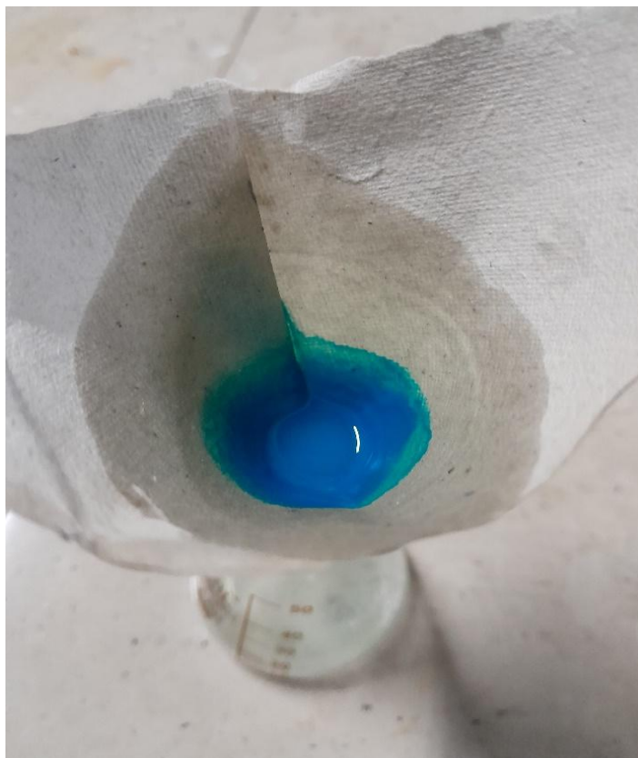
Fig 6 Filtration carried out by simple technique with help of filter paper.
