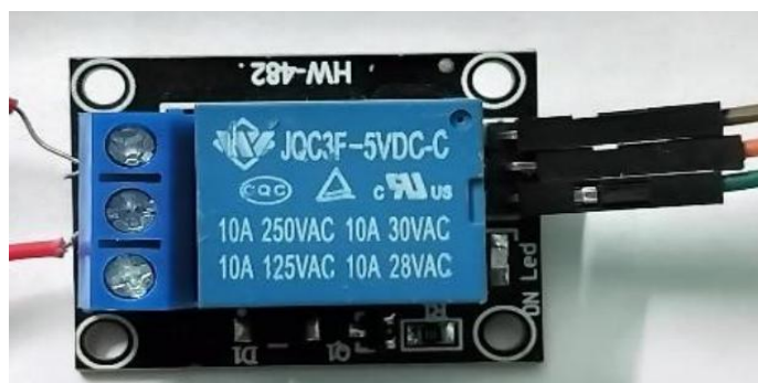
Fig. 3 Relay module (Farnell, Embedded Development Kit, 2022).
