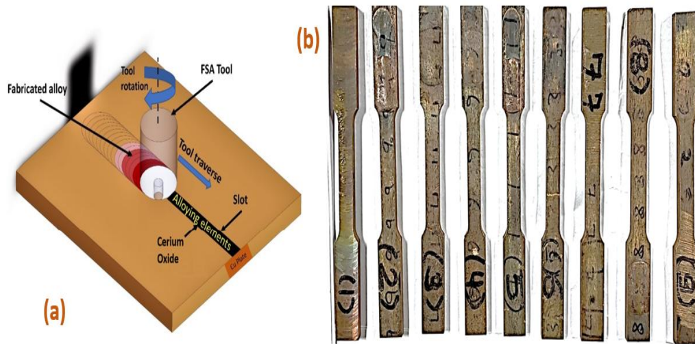
Fig. 3 (a) and (b): Specimens before and after friction-stir processing
