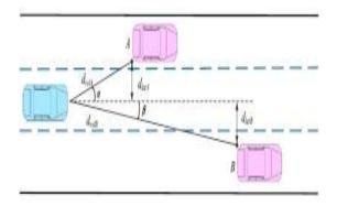
Relative Distance: This refers to measuring the distance between your vehicle and other objects or vehicles on the road. It's crucial for ADAS because knowing the relative distance helps in making decisions related to safety features like adaptive cruise control, collision avoidance, and lane departure warning. Techniques such as radar, lidar, or camera-based systems can be used to calculate relative distances accurately.
