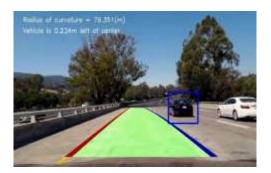
Lane detection is a crucial component of an Advanced Driver Assistance System (ADAS) as it helps in ensuring vehicle safety by alerting the driver when the vehicle deviates from its lane.
