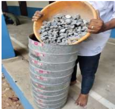
Fig 1: sieve analysis test on coarse aggregate
