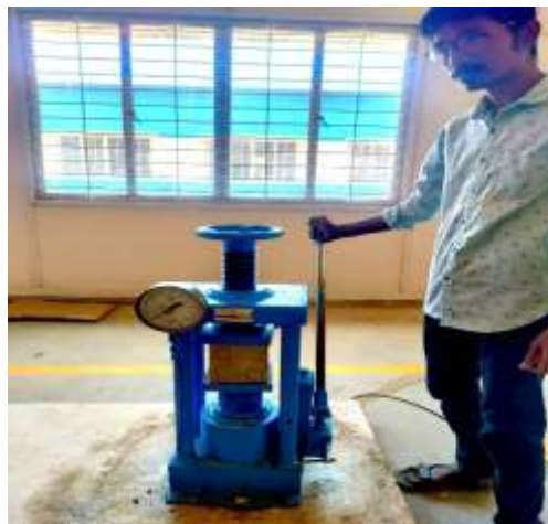
Fig 5: compressive test on concrete
