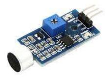
Specification of Sound Sensor: Operating voltage 3.3V-5V
