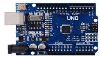
It is the primary component of the framework. In addition, it is an open source microcontroller device with easily accessible software/hardware platform and is compatible with many sensors available. Everything needed for its working is present on the board; we only require a USB cable to directly connect it to the computer or give power using battery source or AC to DC adapter to get started.
