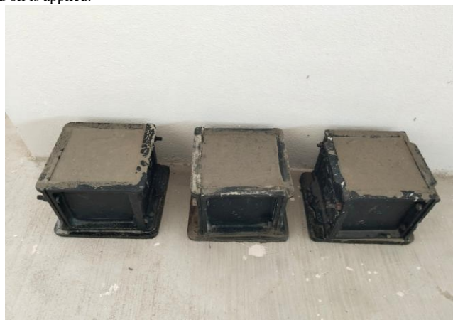
Fig 2: Casting of concrete
