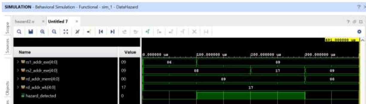
Figure 4.2.10.3 data hazard condition
