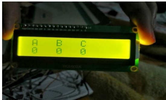
Fig.10 Result on the LCD display when no vote is casted
