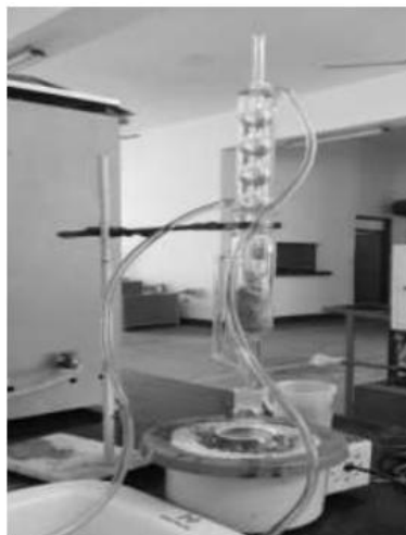
Figure 3 Extraction using Soxhlet Method
