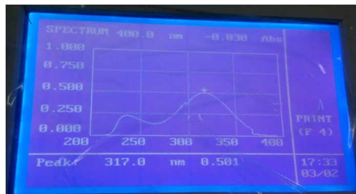
Fig. No. 2 Scanning curve for metronidazole in phosphate buffer (pH 6.8) wavelength range 200nm-400nm
