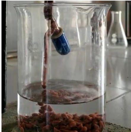
Fig. 11(c). Formation of pellets
